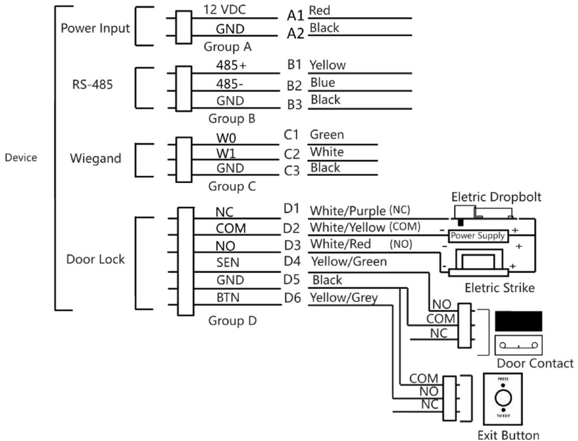
Figure 4-1 Device Wiring
