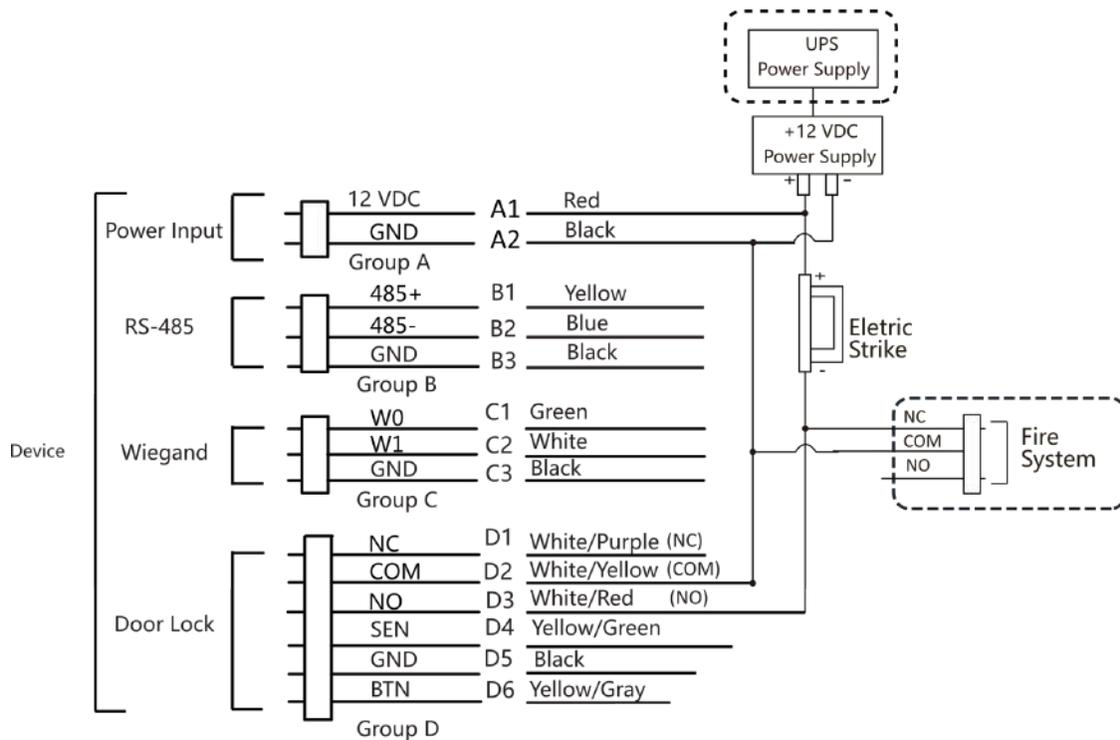
**Figure 4-7 Device Wiring**
