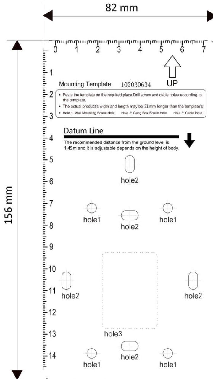
**Figure 3-5 Mounting Template**
