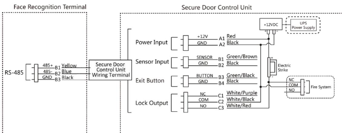
**Figure 4-8 Wiring Diagram**
