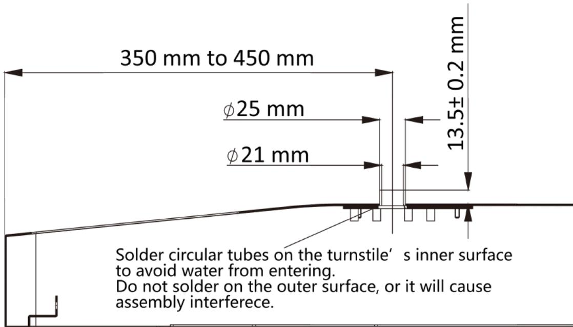
Figure 3-17 Solder Tubes
