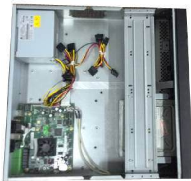
Figure 3-45 Put bracket back
