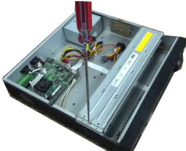
Figure 3-37 Open the top cover
